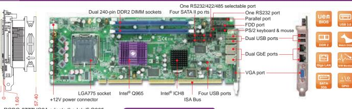
ROBO-8777VG2A adopts the Intel® Q965, ICH8 chipset and Intel® Core™ 2 Duo technologies. It supports DDR2 memory and two Gigabit Ethernet. It's suitable for Digital Signage, Kiosk, and Multimedia applications.
