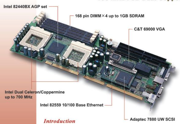
The PEAK 6320A is a full-size single board computer, built with high performance Dual Celeron/Coppermine FC-PGA CPU running 66/100MHz memory Bus, high performance PCI Bus and I/O's, huge memory support, and complies with the new PICMG standard. The PEAK 6320A can run with Dual Intel Coppermine processor up to 700 MHz, memory support up to 1 GB SDRAM.It's the best product with excellent cost/performance ratio for the system integrators in various Mission Critical and heavy-duty applications.
